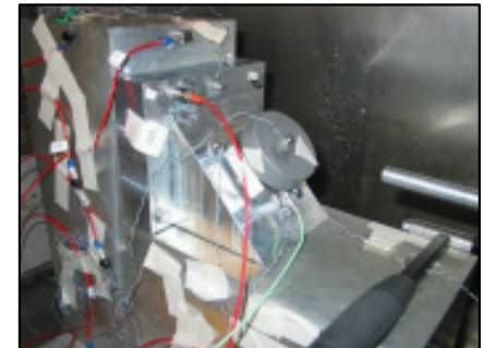
Test article with helium gas gun and rigid load cell – ref [1]
